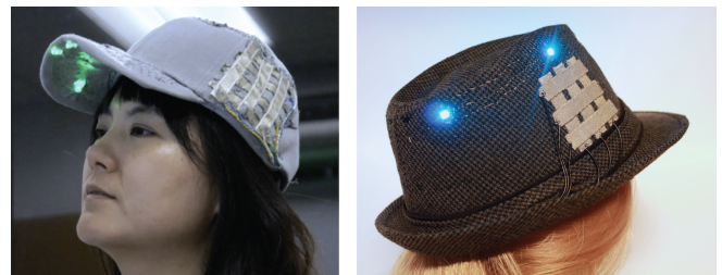
Figure 8. We designed and implemented two different classes of ambient displays. Left: personal under-brim display. Right: public crown display.
